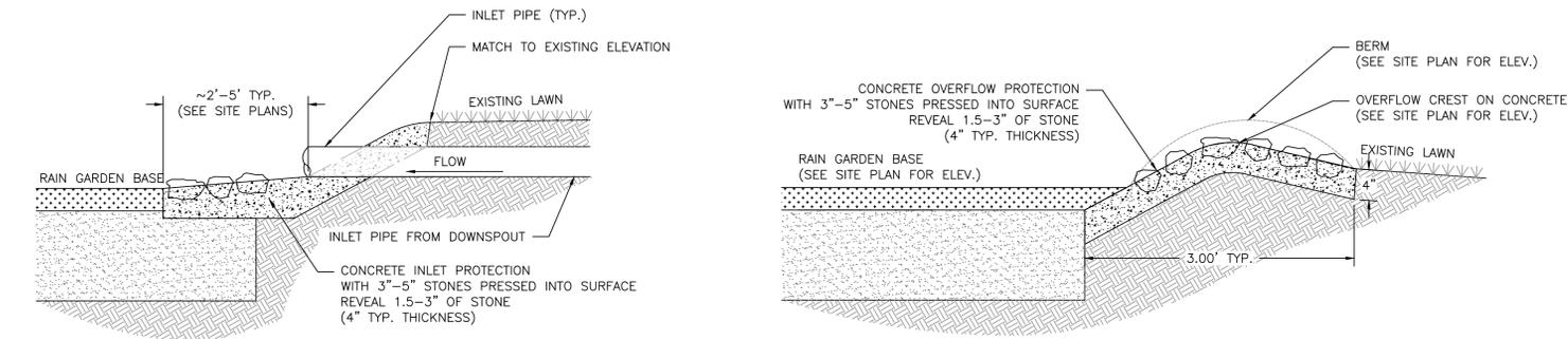
3 INLET PROTECTION CROSS-SECTION
